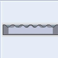
*Unreinforced elastomeric bearing
