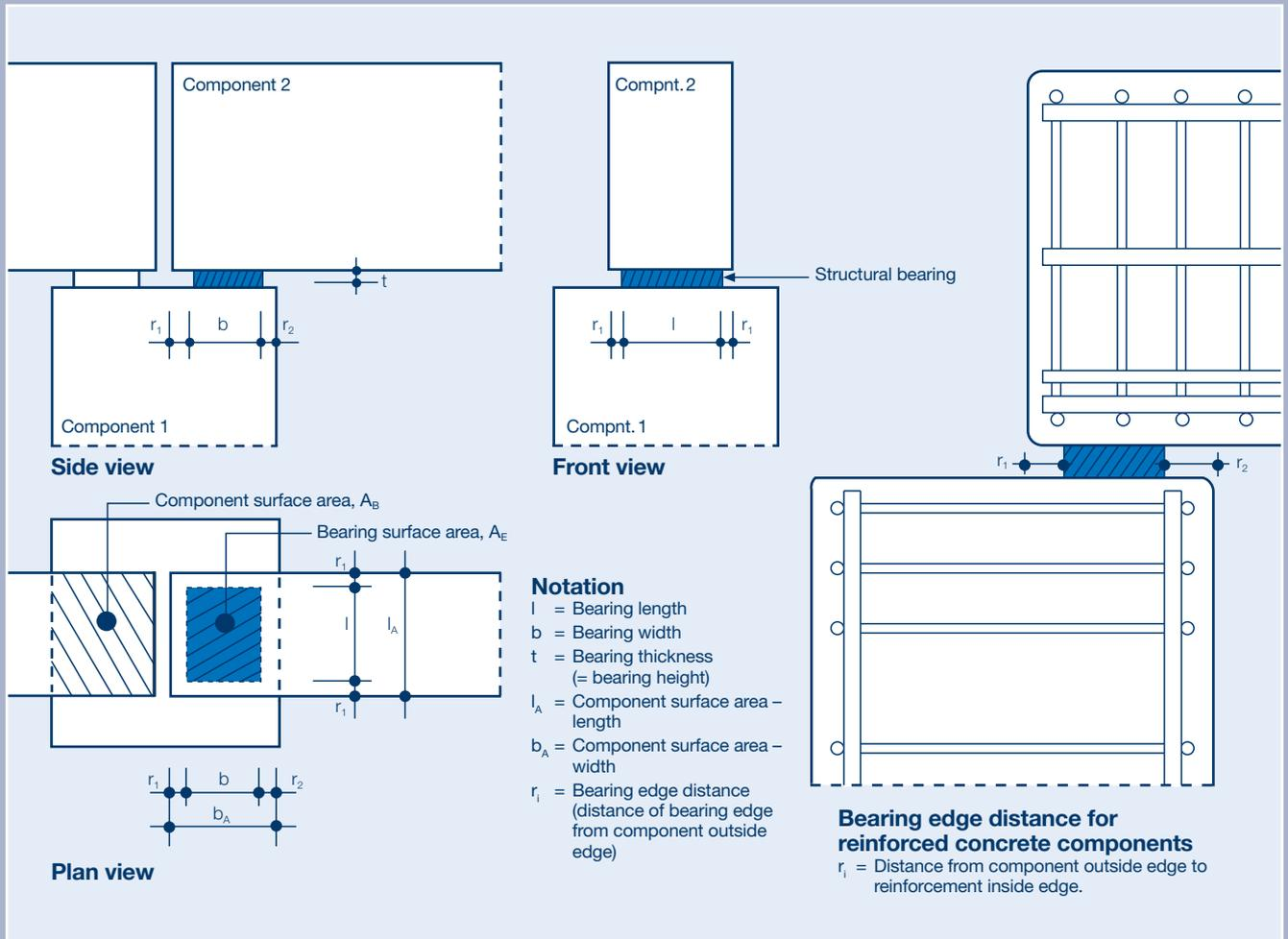
Maximum plan dimensions of an elastomeric bearing for reinforced concrete structures. The provisions of DIN 1045-1 and DAfStb Booklet 525 must be observed. In the case of timber or steel components, the edge distances must be at least 3 cm.
