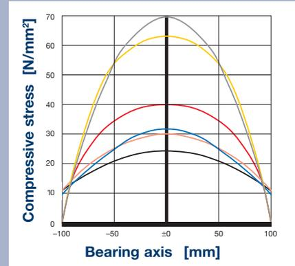
Stress distribution at a bearing joint on the axis of symmetry of the bearing surface of various unreinforced and reinforced elastomeric bearings.
